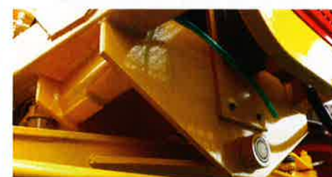
The re-bushed front axle pivot. The steering tract rod is mounted in front of the axle; this track rod required straightening prior to being refitted. (Photo: Jeremy Rowland)
