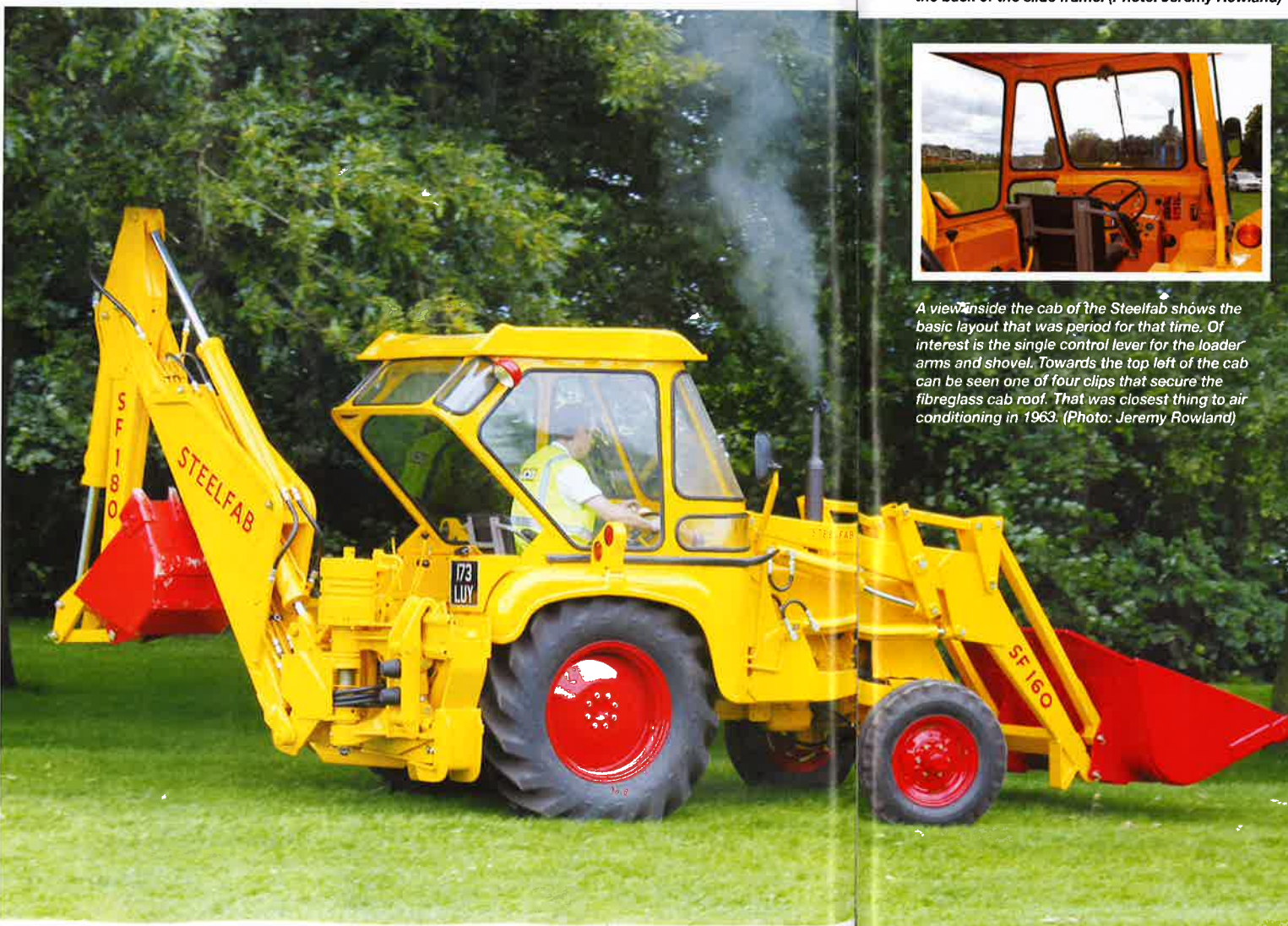
ABOVE: This view shows the digger's backacter and mounting. The rotary actuator that turns the arm is manufactured by Dowty and can be seen between two of the arms operating levers the lower part of the main shaft for this component was re-chromed. The whole arm assembly could slide along the rail and was hydraulically locked into position which was ahead of other competitors' machines at the time. Note the rubber 'bump stops' that prevent the arm from hitting the back of the slide frame. (Photo: Jeremy Rowland)
