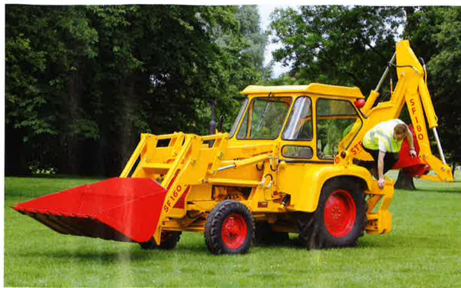
The Steelfab 160/180 has no cab doors and the machine is accessed via a partially open rear cab; the operator climbing in or out in this case next to the backacter. How things have changed! (Photo: Jeremy Rowland)
