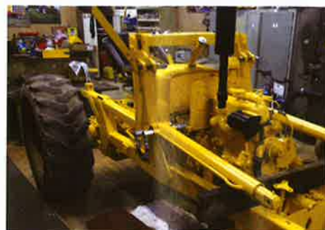
As the restoration progresses the machine slowly starts to take form once again. The re-assembled chassis and skid unit are seen along with the fuel tank, new exhaust and loader arm rams. (Photo: Julian Carder)
