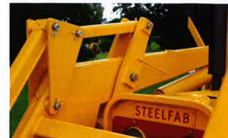
The loader arm linkages that were refurbished with new bushes and linkage pins. The linkage pins on the arms are secured only by a simple split pin. (Photo: Jeremy Rowland)
