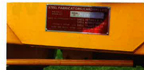
The newly-made manufacturers' plate. It's nice touches like this that really make a restoration job stand out, note the new drag link end on the steering drop arm at the bottom of the picture. (Photo: Jeremy Rowland)
