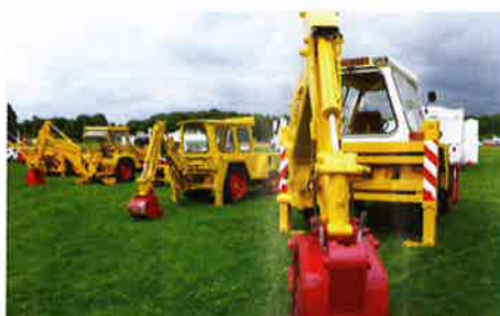
The Steelfab 160/180 has no cab doors and the machine is accessed via a partially open rear cab; the operator climbing in or out in this case next to the backacter. How things have changed! (Photo: Jeremy Rowland)
