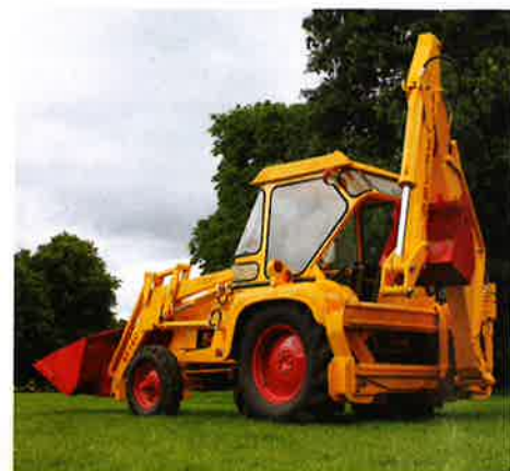
This three quarter rear photograph gives a clearer view of the cab access. The cab itself is secured by only four screw hook type fasteners. (Photo: Jeremy Rowland)
