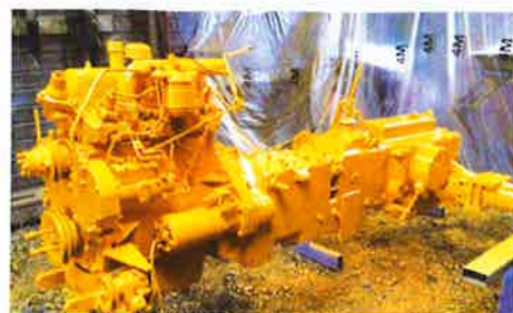
The skid unit stands re-painted ready for assembly to the main chassis. (Photo: Julian Carder)
