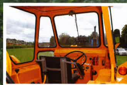
A view inside the cab of the Steelfab shows the basic layout that was period for that time. Of interest is the single control lever for the loader arms and shovel. Towards the top left of the cab can be seen one of four clips that secure the fibreglass cab roof. That was closest thing to air conditioning in 1963. (Photo: Jeremy Rowland)
