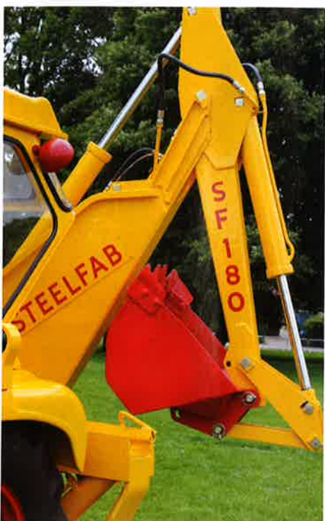
A close-up shot of the boom and dipper arm. Of interest are the square mounting linkage pins for the pivots and hydraulic rams. All of the pins on this digger have been newly manufactured. (Photo: Jeremy Rowland)
