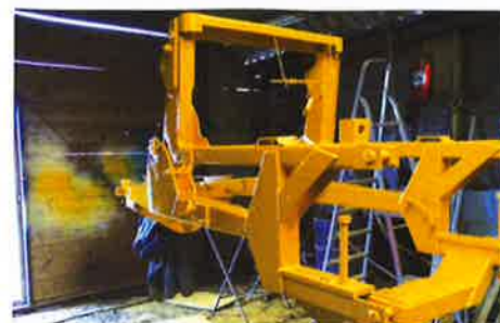
The chassis is repainted after shot-blasting. Supporting the chassis in this way enables better access to ensure that every part is evenly covered with paint. (Photo: Julian Carder)
