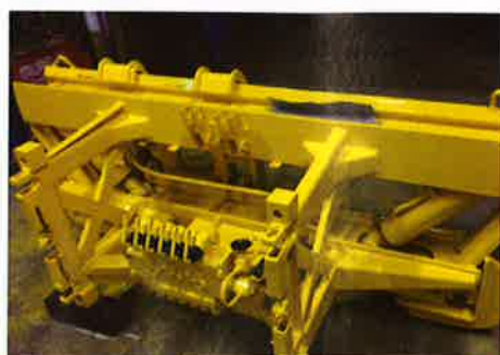
The backer frame along with the stabiliser legs and hydraulic control valve are ready for fitting back onto the digger. (Photo: Julian Carder)
