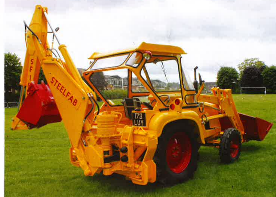
ABOVE: This view shows the digger's backacter and mounting. The rotary actuator that turns the arm is manufactured by Dowty and can be seen between two of the arms operating levers the lower part of the main shaft for this component was re-chromed. The whole arm assembly could slide along the rail and was hydraulically locked into position which was ahead of other competitors' machines at the time. Note the rubber 'bump stops' that prevent the arm from hitting the back of the slide frame. (Photo: Jeremy Rowland)
