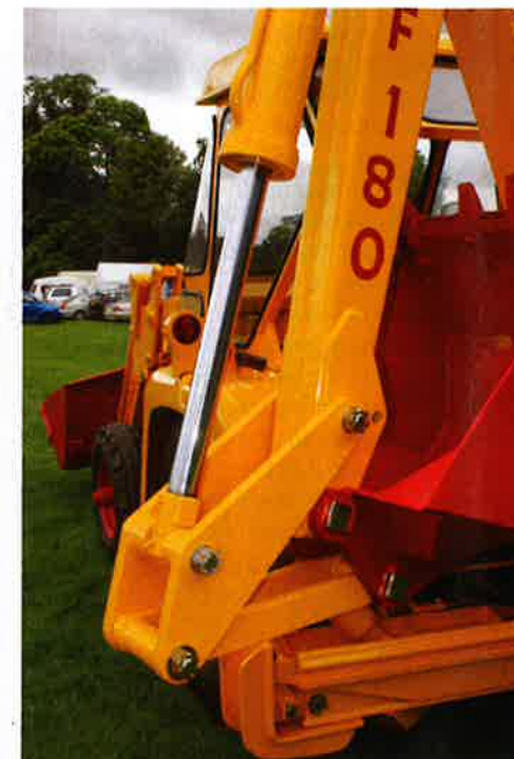
The bucket pivot and ram detail show that the square linkage pins are secured on the other side by a castle nut and split pin albeit the split pins are missing in this instance. (Photo: Jeremy Rowland)
