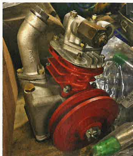
Left: The air compressor, hand valve and release valve removed ready for reconditioning Right: Fully rebuilt and waiting to be refitted to the Fordson tractor, the air compressor for the braking system is belt-driven directly off the transmission (Photos Julian Carder)
