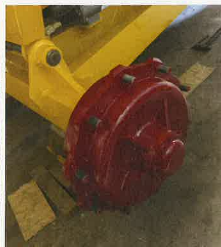
Left: The left-hand new wing has been fitted into position and the cab is being jugged ready to get it into position; note the Poole hitch that can be seen here bolted to the underside of the tractor's drive axle Middle: The repaired cab frame sits on the two newly fitted wings Right: The trailer's offside brake drum and hub assembly refitted and painted as the restoration progresses (Photo Julian Carder)
