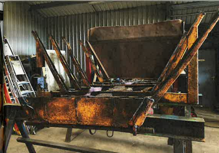
◀ The poor condition of the dumper body is evident in this photo; the bottom of the body had rotted into holes and the main support ribs and cross members were also badly corroded (Photo Julian Carder)
