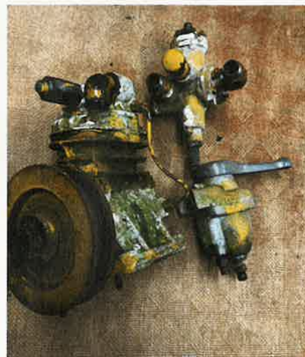
Left: The air compressor, hand valve and release valve removed ready for reconditioning Right: Fully rebuilt and waiting to be refitted to the Fordson tractor, the air compressor for the braking system is belt-driven directly off the transmission (Photos Julian Carder)
