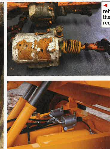
Beneath the tilted dumper body you can see the two refurbished air brake cylinders and beneath the closest one is the compressed air reservoir mounted out of sight in the chassis 'A' frame. (Photo Jeremy Rowland)
