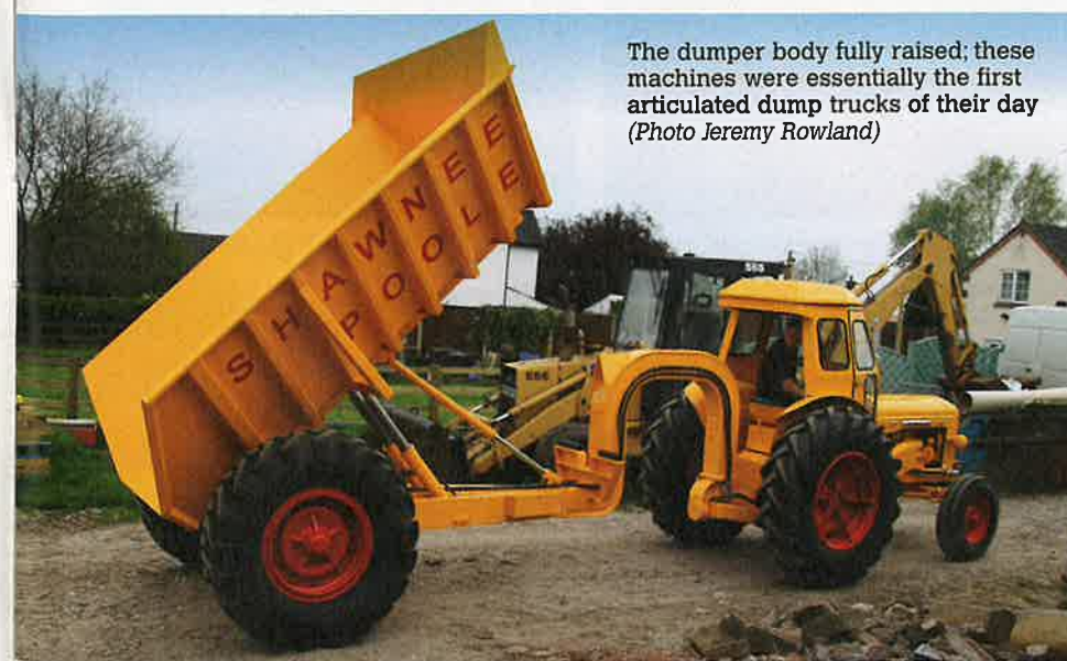
This nearside view of the dumper gives a clearer view of the Poole hitch bolted underneath the tractor's drive axle (Photo Jeremy Rowland)
