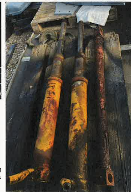
◀ Awaiting strip down, shot blasting then refurbishment are the two air brake cylinders; the mechanical side of the brakes also required much attention (Photo Julian Carder)
