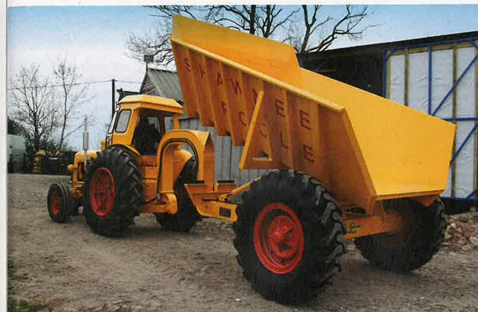
This nearside view of the dumper gives a clearer view of the Poole hitch bolted underneath the tractor's drive axle (Photo Jeremy Rowland)
