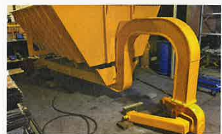
Most of the work on the trailer has now been finished; the Poole hitch has been placed facing backwards in this photo, but the two ends of the fork are bolted underneath the tractor's drive axle to give maximum tractive effort (Photo Julian Carder)
