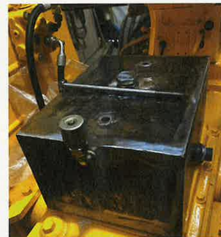
Left: The newly designed and fabricated hydraulic oil tank rests in position; the driver's seat will later be attached to the top of this tank. The tipper control spool valve is visible in the top left of the photo Right: Finally, the hydraulic oil tank is finished with the driver seat fastened to it (Photos courtesy of Julian Carder)
