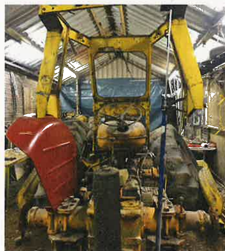
Left: The left-hand new wing has been fitted into position and the cab is being jugged ready to get it into position; note the Poole hitch that can be seen here bolted to the underside of the tractor's drive axle Middle: The repaired cab frame sits on the two newly fitted wings Right: The trailer's offside brake drum and hub assembly refitted and painted as the restoration progresses (Photo Julian Carder)
