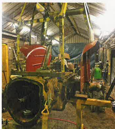
Left: The left-hand new wing has been fitted into position and the cab is being jugged ready to get it into position; note the Poole hitch that can be seen here bolted to the underside of the tractor's drive axle Middle: The repaired cab frame sits on the two newly fitted wings Right: The trailer's offside brake drum and hub assembly refitted and painted as the restoration progresses (Photo Julian Carder)
