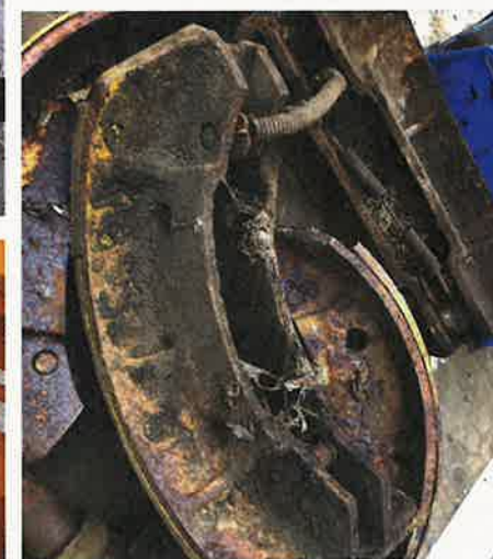
The worn trailer brake shoes; much money and effort were spent getting the brakes working properly and to 'as new' condition (Photo Julian Carder)
