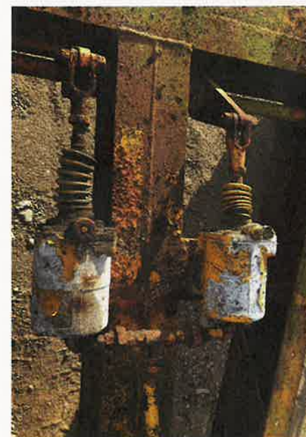
Looking down on top of the trailer 'A' frame, the two air brake cylinders can be seen along with the actuating arms which operate 'S' cam type brakes (Photo Julian Carder)
