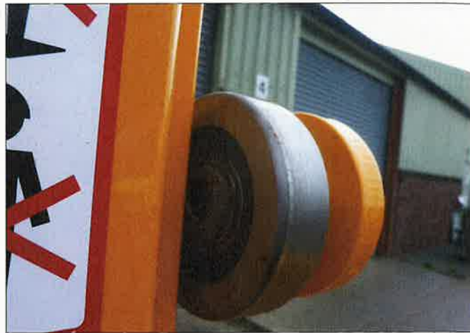
One of the many supporting roller bearings that were replaced on the forklift's mast. (Photo Jeremy Rowland)
