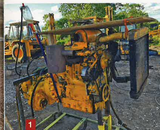
1: The engine and transmission unit mounted on a stand with a temporary fuel feed for testing; these did not require much attention short of cleaning down and painting 2: Hydraulic rams and main spool valve cleaned down ready for reconditioning and painting 3: The partially stripped mast; numerous roller bearings were replaced on the mast, the main lift rams were fully reconditioned, the lifting chain was not worn beyond its safe limit (Photo Julian Carder) 4: The bare chassis shot-blasted and given a first coat of primer. (Photo Julian Carder)
