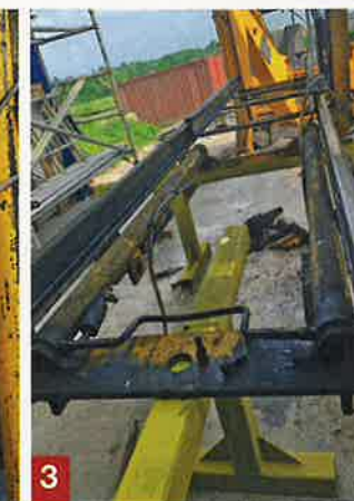
1: The engine and transmission unit mounted on a stand with a temporary fuel feed for testing; these did not require much attention short of cleaning down and painting 2: Hydraulic rams and main spool valve cleaned down ready for reconditioning and painting 3: The partially stripped mast; numerous roller bearings were replaced on the mast, the main lift rams were fully reconditioned, the lifting chain was not worn beyond its safe limit (Photo Julian Carder) 4: The bare chassis shot-blasted and given a first coat of primer. (Photo Julian Carder)
