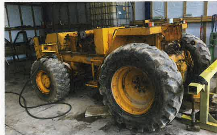
Left: The JCB 930 with the fork mast removed as the strip down of the machine commences in earnest
