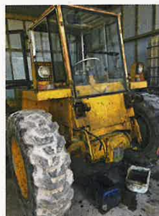
Left: The JCB 930 with the fork mast removed as the strip down of the machine commences in earnest
