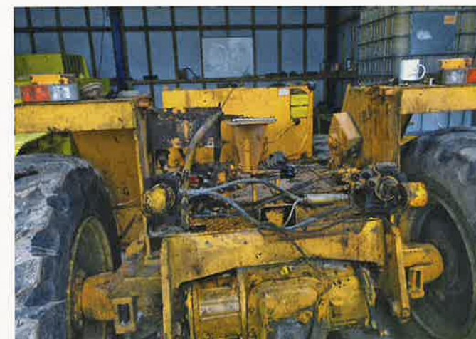
◀ This frontal view shows the progression of the strip down; the main hydraulic spool valve lies on the cab floor while the cab electrical connections can be seen resting on the nearside fork tilt ram (Photo Julian Carder)
