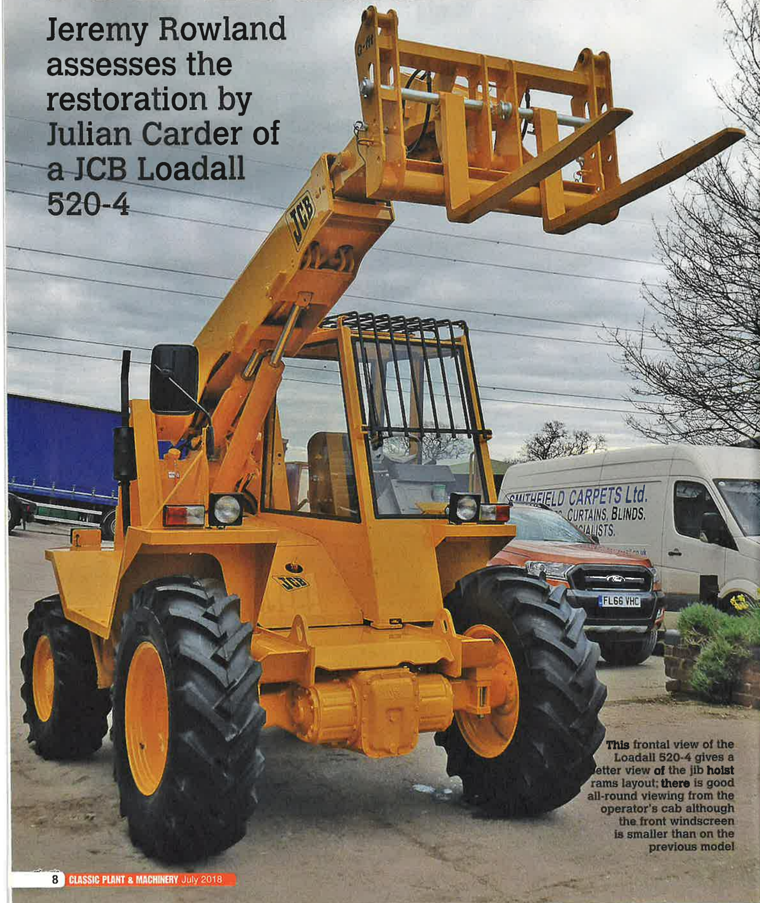
Unlike the early version, the 520-4 has the jib hoist rams mounted in-line with each other; whereas they are parallel to each other on the old 520
