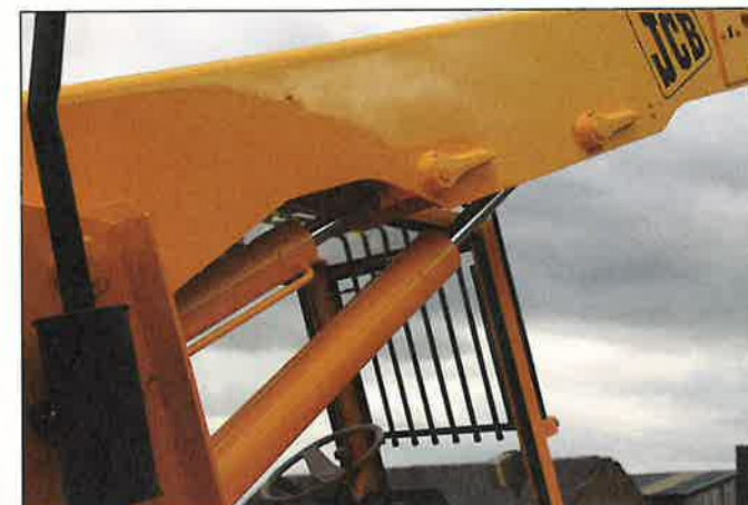
Unlike the early version, the 520-4 has the jib hoist rams mounted in-line with each other; whereas they are parallel to each other on the old 520
