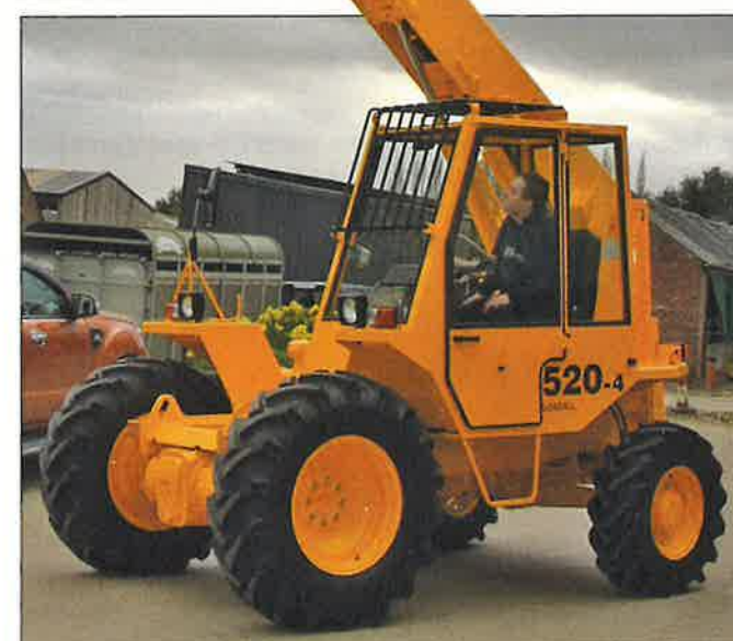
Julian displays the Loadall's height and reach; having a good reach and lifting height along with excellent vision of the load made the Loadall more flexible than other types of machinery used for similar purposes
