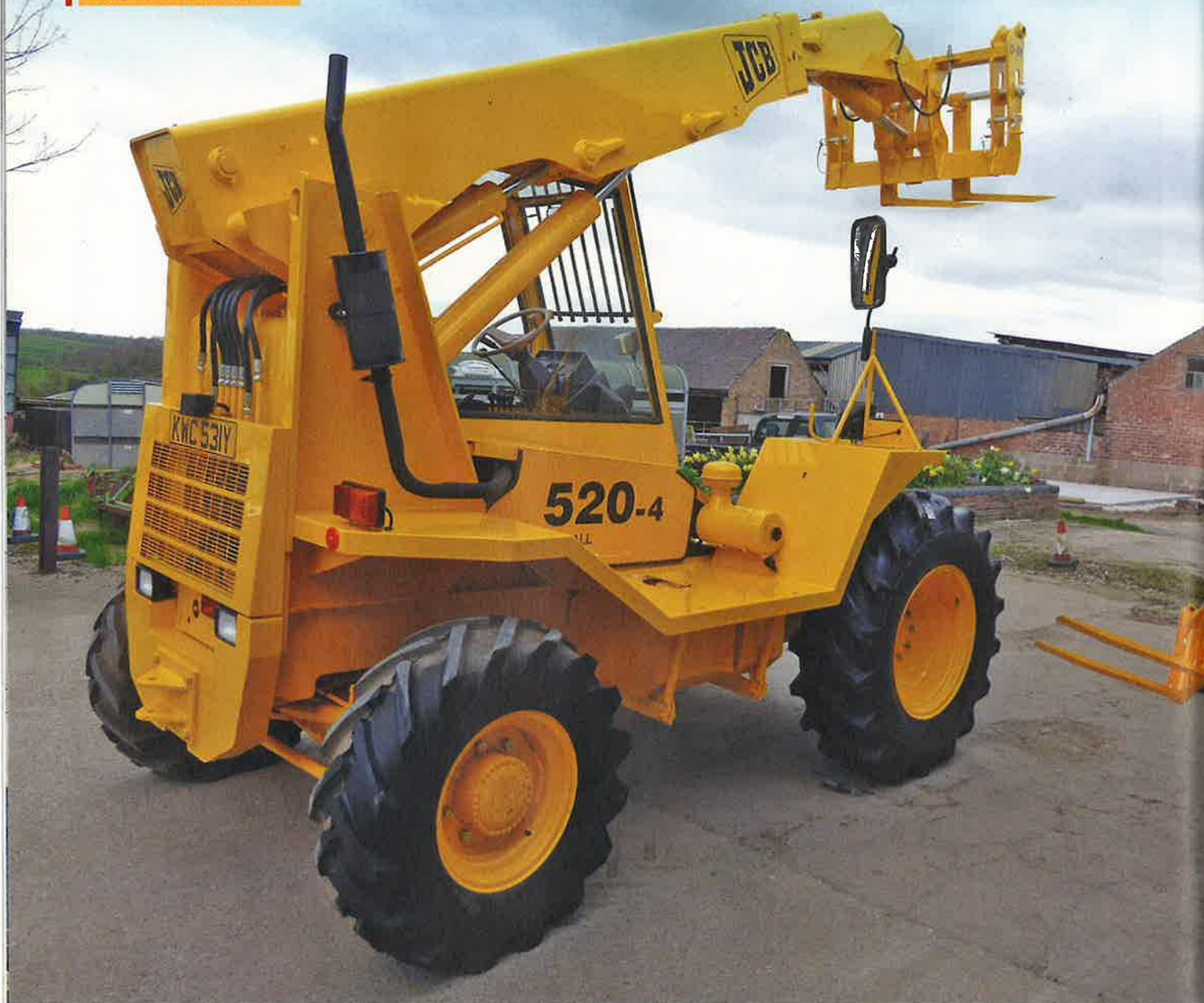
An offside view of the Loadall. Note the exhaust pipe that runs to the silencer mounted on the jib support. The pipe was completely fabricated from new as stock parts were no longer available
