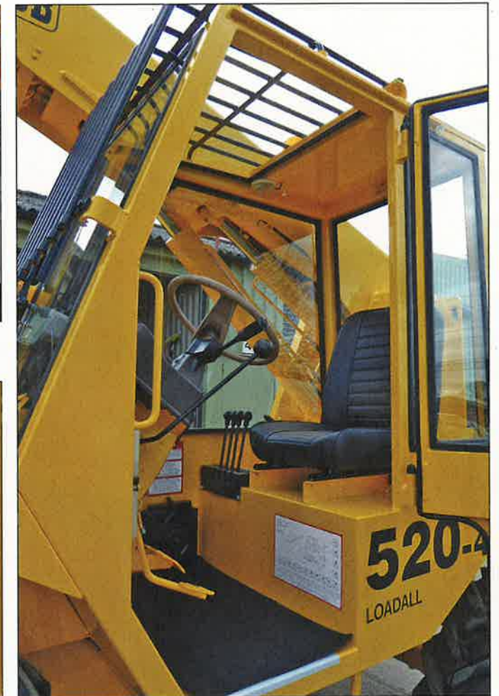
Peering into the refurbished Loadall cab that looks like it's brand new; the four-control levers for operating the jib functions are more ergonomically placed than in the original 520 telehandler
