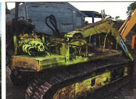
Left: Within a week of being unloaded the Hymac was already well stripped in this photo supplied by Julian Carder Right: A rear shot of the upper works with the rear counterweight removed; note the old dynamo fitted to this machine, no alternator here (Photo courtesy Julian Carder)
