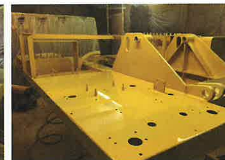
Left: A rear photo of the upper platform painted and ready for fitting back on the excavator (Photo courtesy Julian Carder)
