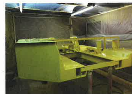
Left: A rear photo of the upper platform painted and ready for fitting back on the excavator (Photo courtesy Julian Carder)
