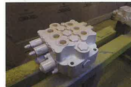
Left: A close up of one of the three spool valves fitted to all of Hymac's 580 machines, these are connected by control rods to the operator's control levers in the cab Middle: The undercarriage in the paint booth with the undercoat applied; the Staffa motor and slew ring have also been fitted, the motor rotates the machine's upper works when the slew function is operated Right: Peering inside one of the two track drive gearboxes after refurbishment, on occasion these gears have been known to fail on older machines
