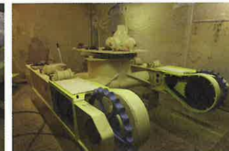
Left: A close up of one of the three spool valves fitted to all of Hymac's 580 machines, these are connected by control rods to the operator's control levers in the cab Middle: The undercarriage in the paint booth with the undercoat applied; the Staffa motor and slew ring have also been fitted, the motor rotates the machine's upper works when the slew function is operated Right: Peering inside one of the two track drive gearboxes after refurbishment, on occasion these gears have been known to fail on older machines
