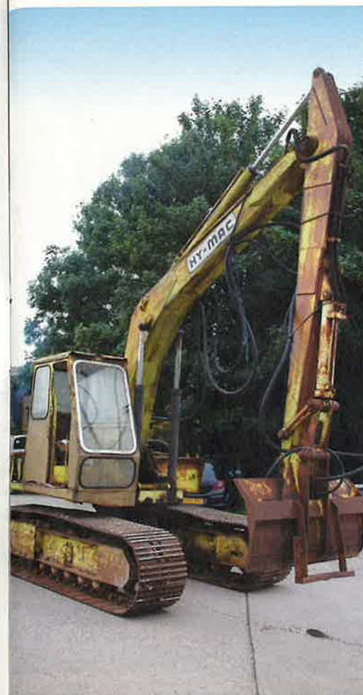
This offside view of the machine shows the rot along the bottom of the cab, quite normal for a machine that is now fifty years old
