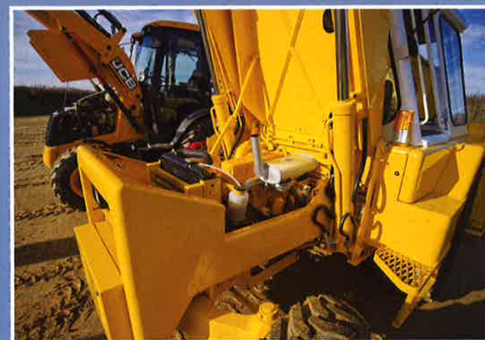
Above and Above Right: The Leyland engine delivers 70hp backed up by 258Nm of torque at 1300rpm, compared with the ultra-modern JCB motor rated at 91hp and 433Nm of torque at 1400rpm.
